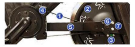
4. Remove the rear belt pulley finger guard 4 by removing the fasteners (2x) using a 5 mm hex key. Retain fastener hardware for installation.
